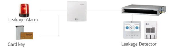
Refrigerant Leakage Detection Alarm
